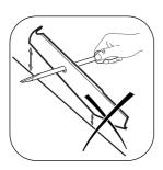
If the cutterblade is not balanced the heavy end will rotate downwards. Sharpen the heavy end until the cutterblade is correctly balanced.
